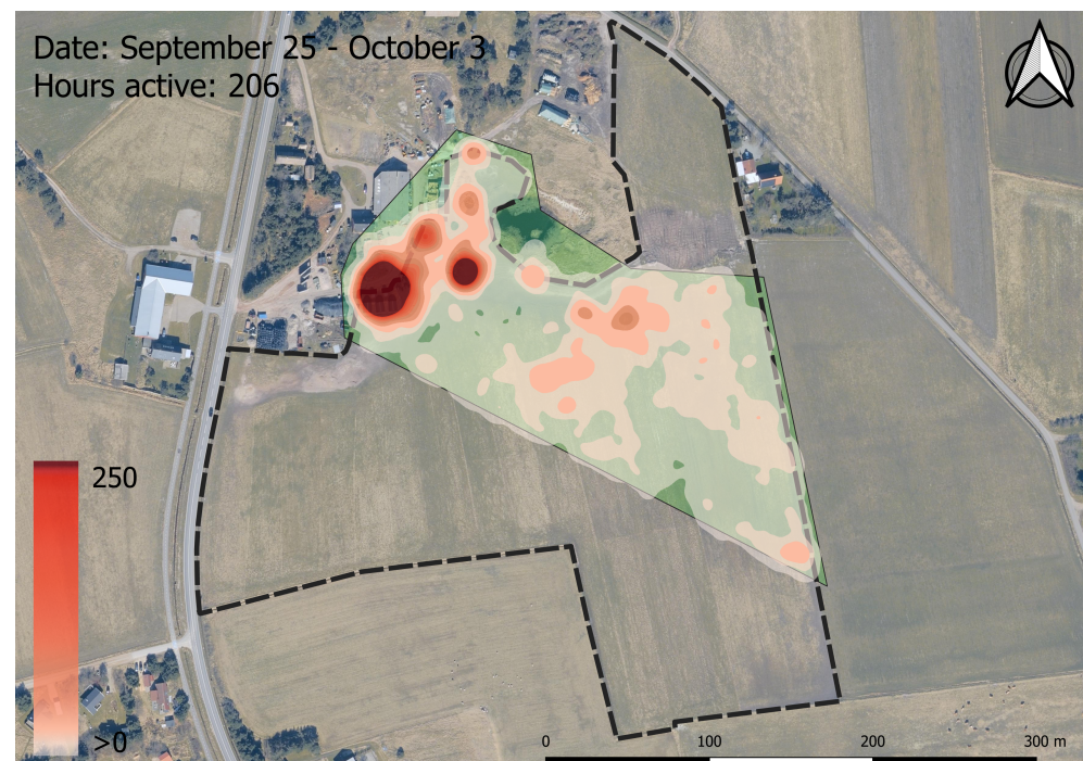
Figure 2. Heatmap visualising all Poll messages sent during the period from 25 September to 3 October. The green area shows the virtual enclosure area to which the bull calves were limited. The white to red colour scale indicates the number of Poll messages within a 10 m radius on a discrete scale, ranging from 1 point to above 250 points. The coordinates of the upper left corner of the map frame are 55°25′23.131″ E 8°23′53.531″ N. Contains data from the Agency for Data Supply and Infrastructure, Forårsbilleder Ortofoto-GeoDanmark, December 2022.
