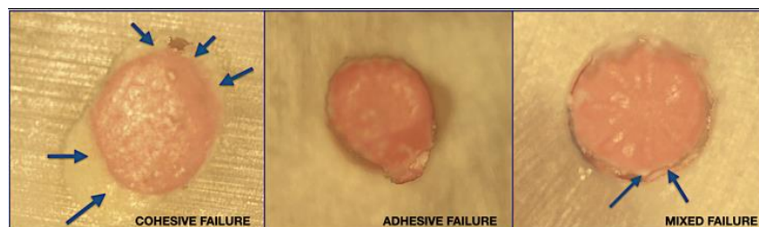
Figure 2. Samples under magnification \times 20 as observed just after push-out test illustrating the three possible bond failures. The push out test stops automatically after decohesion of the gutta-percha cone. The latter is nevertheless still visible on the pictures due to its incomplete dislodgment. The blue arrows indicate some areas showing the sealer.
