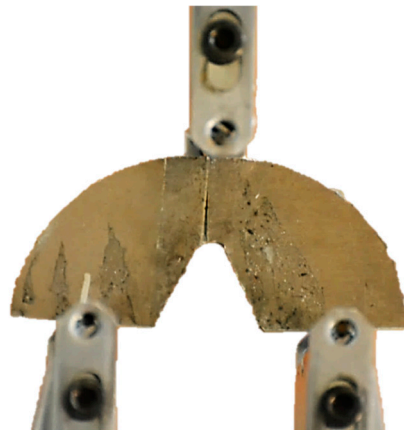
Figure 3. SCB notched sample under pure mode I fracture test.
