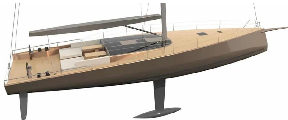
Figure 17. Baltic yachts made from flax-fibre-reinforced composites (source: https://www.metstrade.com/news/construction-and-material/flax-basalt-fibres-future-marine-composites/ , 5 July 2020) [261].
