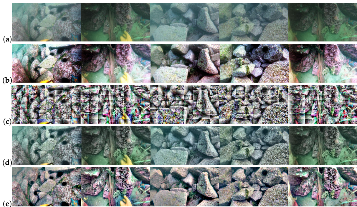
Figure 5. Comparison of underwater image enhancement results for different algorithms: (a) original images; (b) HE; (c) AHE; (d) CLAHE; (e) MSRRCR.
