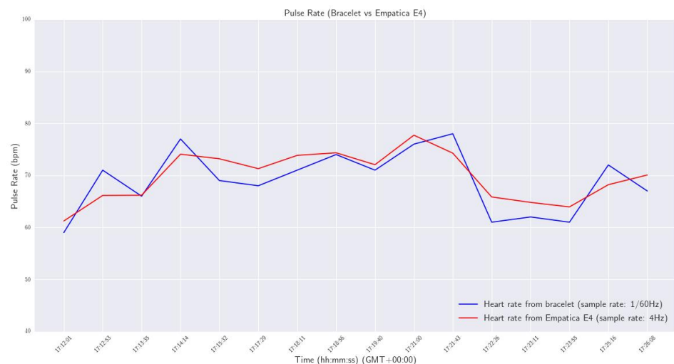
Figure 9. Pulse Rate - Smart wristband vs Empatica E4.
