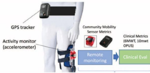
A) Accelerometer can be combined with GPS devices to track how and where a person moves. Adapted from Lonini et al., 2021.
