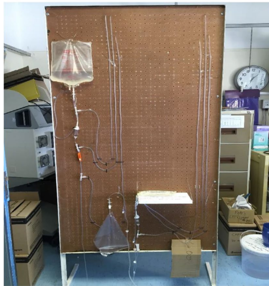
Fig. 1 Set-up of in vitro experiments of gravity-assisted CFPD. Manometers inserted along the line at several points to measure pressure at different flow rates, the height of delivery and collection bags and during constriction of in and out flow. Drip chambers used to measure the flow rate
