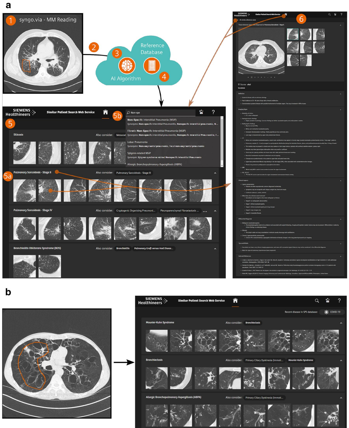
Figure 2. (a) Schematic Illustration of the Similar Patient Search Web Service. (1) The user selects an ROI on an axial CT slice using the host Application ( syngo.via VA40A). The slice, along with the ROI, is sent to the cloud service (2). A deep-learning-based feature representation (fingerprint) for the slice/ROI combination is computed in the cloud (3). The fingerprint is then compared to pre-generated fingerprints from the reference database (4). The tool returns a webpage that shows the most similar image patches from the reference database and their corresponding diagnosis (5). The clinical reference content from Thieme is accessible by a single click on the disease detail page (6). (b) Example SPS result from the study: Left: Input Slice (case with Mounier Kuhn Syndrome) with the ROI chosen by the study participant (orange outline) Right: SPS User interface with top 3 results of the similarity search for this case.
