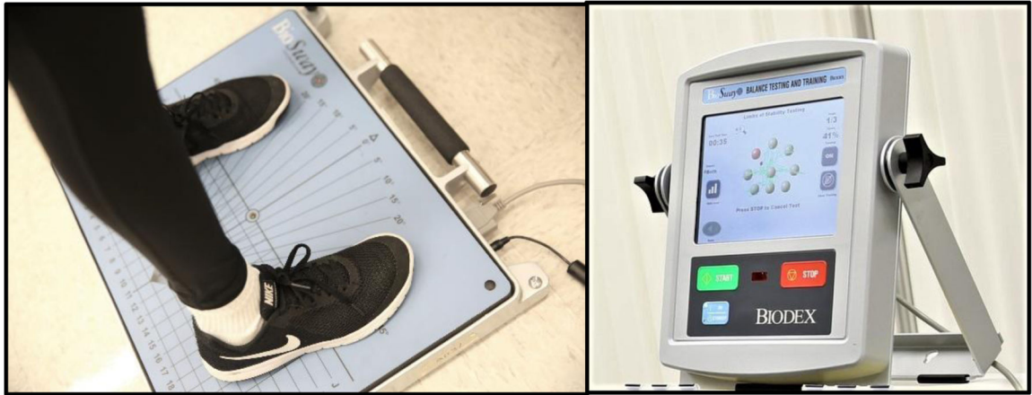
Figure 1. Participant standing on the portable BioSway force plate ( left ) and the BioSway computer displaying the Limits of Stability Task ( right ).
