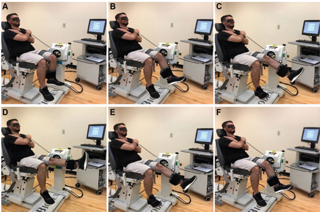
Figure 1. Top row: JPS test in extension. (A) Starting angle (90° of flexion). (B) Target angle (60° of flexion). (C) Target angle (30° of flexion). (B) and (C) were randomly ordered. Bottom row: JPS test in flexion. (D) Starting angle (0° of flexion). (E) Target angle (30° of flexion). (F) Target angle (60° of flexion). (E) and (F) were randomly ordered. JPS, joint position sense.
