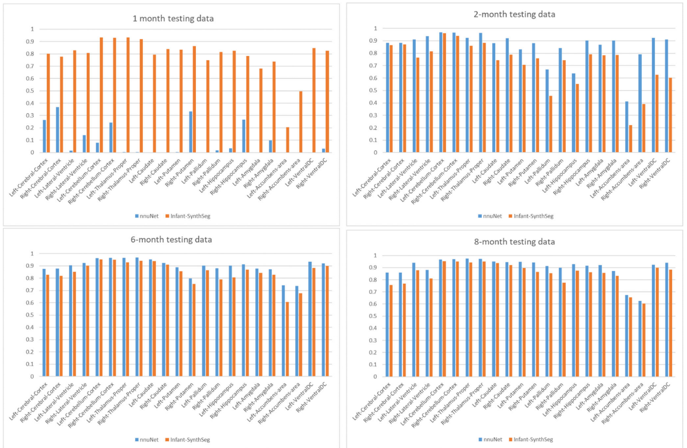
Figure 4: Dice score: SynthSeg-infant (SynthS) vs nnU-Net (NNU), each 1 subject at 1, 2, 6, 8 months. While nn-UNet fails at 1 month, it overall performs at a similar or better level for the other ages.
