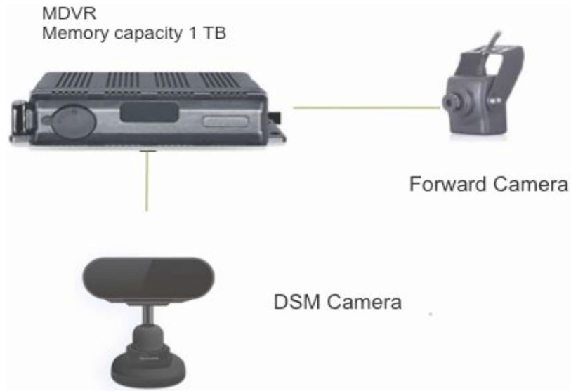
Figure 12. The architecture of the video system.
