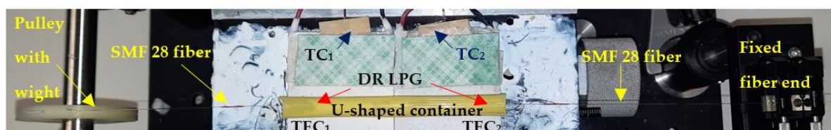
Figure 5. Experimental jig: the DR LPG spliced between two SMF 28 fibers was placed in a U-shaped container (yellow), which was placed on two thermoelectric coolers, TEC 1 and TEC 2 , mounted on a heat sink covered with thermoconductive paste (white) and upon which were fixed two thermocouples, TC 1 and TC 2 .
