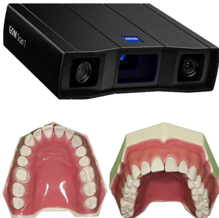
Figure 4. The master model was scanned with an industrial high-resolution reference scanner to obtain a highly accurate digitized reference model GOM Scan 1 (GOM, Zeiss Group, Braunschweig, Germany).
