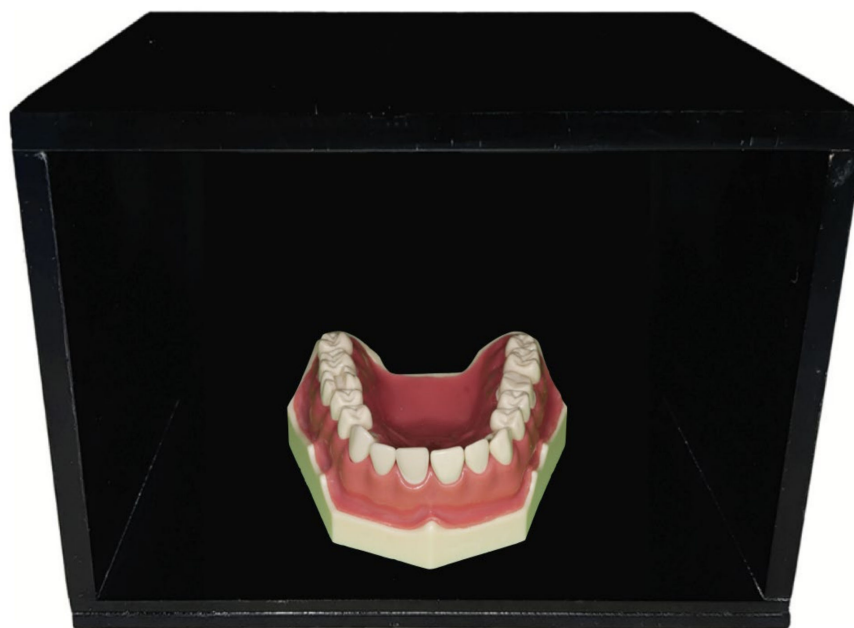
Figure 1. The epoxy-resin-made maxillary dental arch was inserted in an opaque black methacrylate box, in order to simulate oral cavity.
