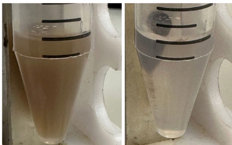
Figure 3. Magnetic separation of \text{Fe}_3\text{O}_4@/\text{CaCO}_3 nanocomposite (0.45 mg/mL of \text{Fe}_3\text{O}_4 synthesis) immediately (left) and after 15 s (right).
