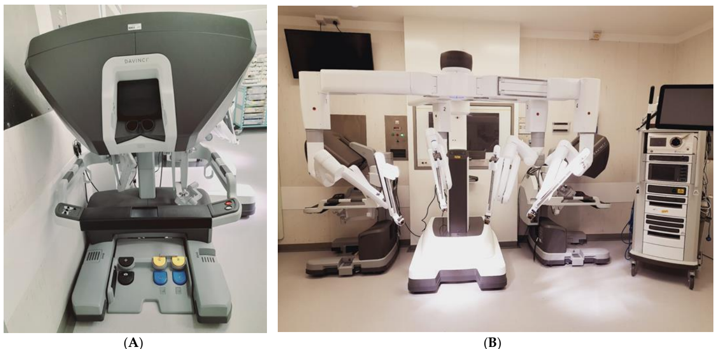
Figure 1. Da Vinci Xi Robotic System (A) Surgeon's Console. (B) Robot cart with 4 arms deployed in centre of image, the vision cart is to the right of the image.
