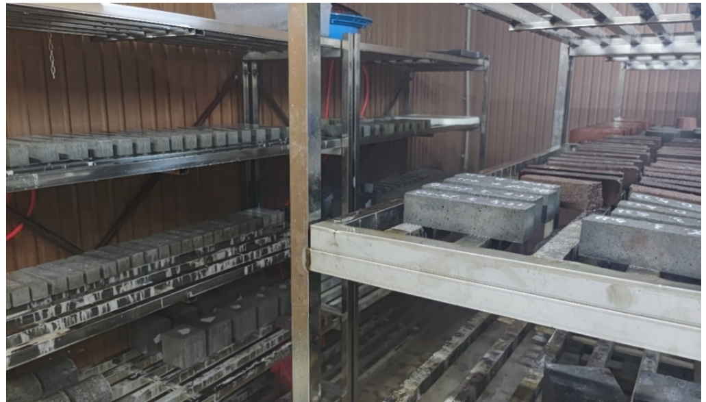
Figure 3. Specimens were cured for 7 days and 28 days in the standard curing room.
