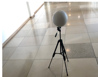
Figure 5. The sphere target is made of plastic with a special matt-textured varnish. It also has a removable magnetic base (M8 thread).
