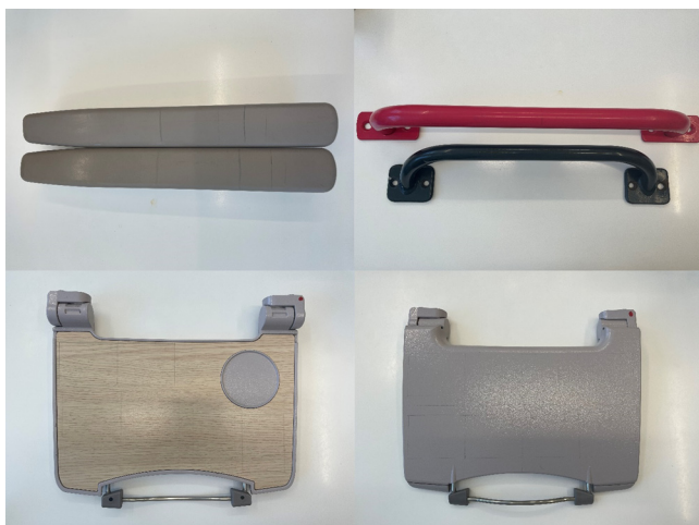
FIG 3 Top left, Terluran 22 arm rests; top right, plastic coated hand poles; bottom left, HPL tray table (Side A); bottom right, CSS tray table (Side B).
