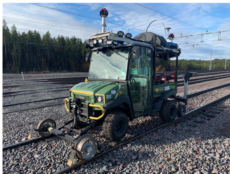
Figure 6. Mobile mapping system for tunnel inspections developed by the company WSP [38].
