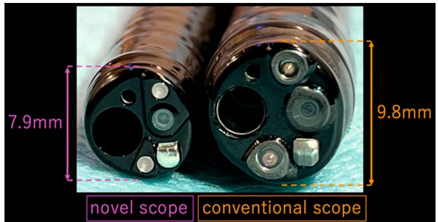
▶ Fig. 1 Comparison of outer diameter of the novel scope and the conventional treatment scope. The novel scope has a thinner outer diameter of 7.9 mm, whereas the conventional therapeutic scope has an outer diameter of 9.8 mm.
