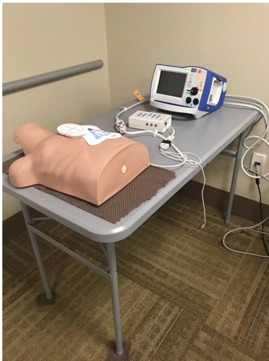
Fig. 2 – Setup showing the CPR manikin, portable table, nonslip material under the manikin and front table legs, and Zoll Series R Defibrillator on the table.
