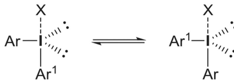
FIGURE 4. Exchange of axial and equatorial aryl ligands in diaryliodonium salts through pseudorotation
