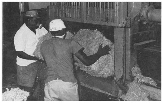
FIG. 2. Bale being loaded for compression.
