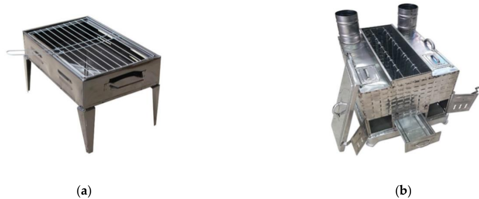
Figure 1. The photographs of the barbecues used in the current study. (a) Traditional barbecue for the direct method; (b) custom-made barbecue for the indirect method.
