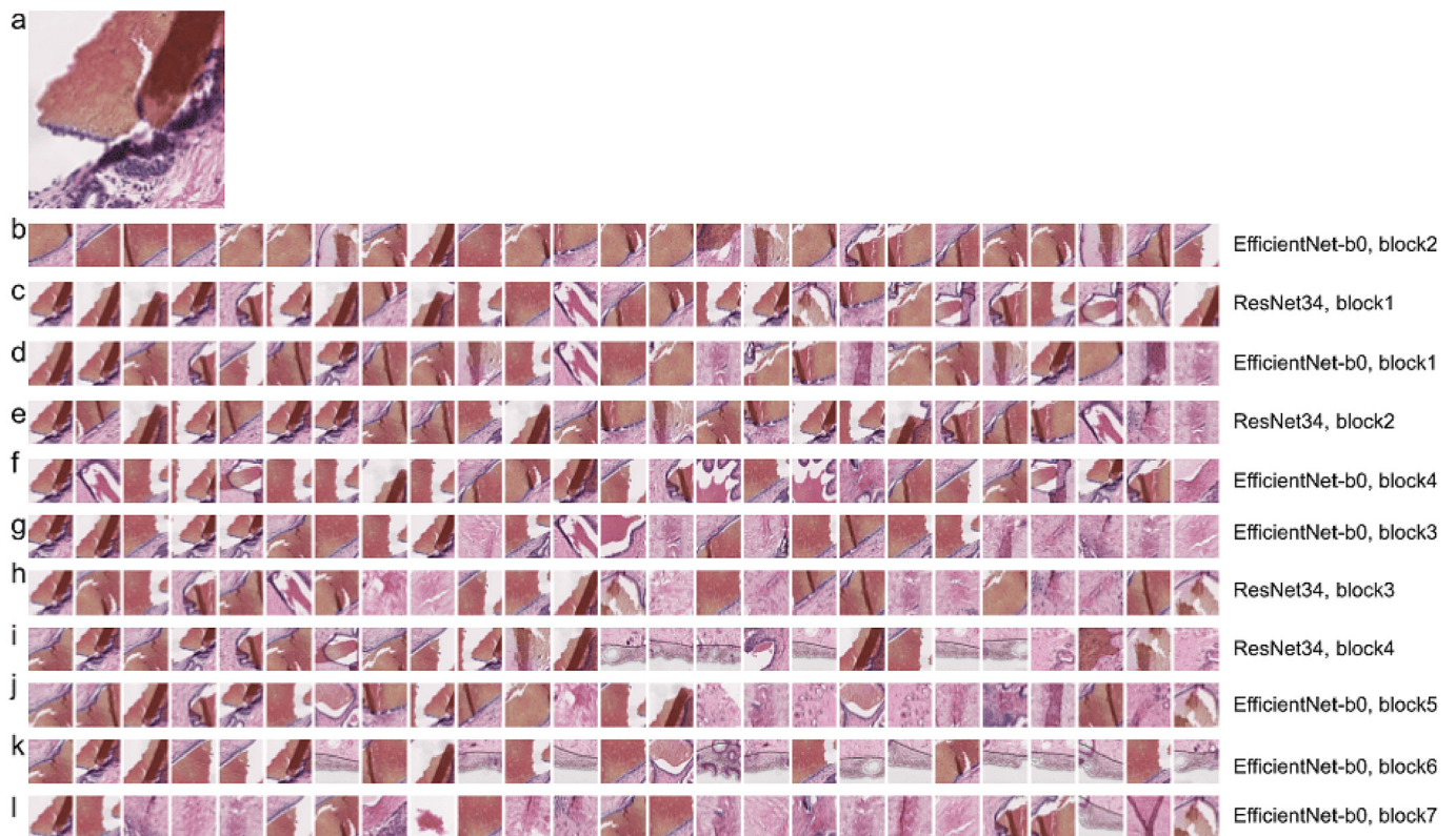
Fig. 11. Visual comparison of Imagenet pre-trained features of ResNet-34 and EfficientNet-b0. (a) Shows a reference image. Each row contains 25 patches with minimum distance from a reference patch. Rows of patches are sorted in order of semantically most similar (row b) to least similar (row l). Row (b) corresponds to patches extracted from EfficientNet0-block-2. Similarly, row (c) to (l) corresponds to features extracted from ResNet34-block-1, EfficientNet-b0-block-1, ResNet34-block-2, EfficientNet-b0-block-4, EfficientNet-b0-block-3, ResNet34-block-3, ResNet34-block-4, and block 5 to 7 of EfficientNet-b0, respectively.
