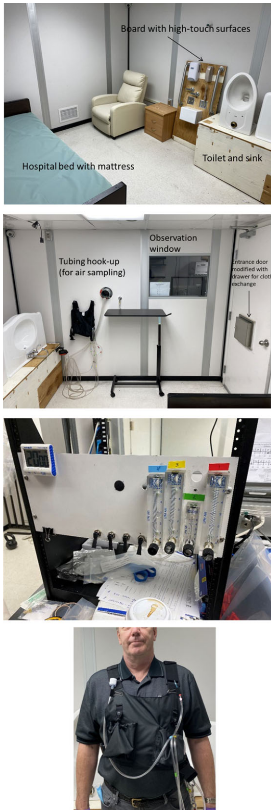
Fig. 1. Chamber configuration and equipment at the Monell Chemical Senses Center. Top 2 photos: Environmental chamber configuration with furniture and high-touch surfaces, sample tubing hook-up, and chamber entrance door, which was modified with a drawer for cloth exchange. Third from top: Sample collection manifold constructed with 4 key instrument rotameters and a Gast DOA P707-AA vacuum pump. Bottom: Customized sampling vest, with Tygon tubing from the 4-channel sample collection manifold to the breathing zone of the volunteer and connected to the sample cartridges.
