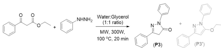
Scheme 1. Microwave assisted synthesis of 1,3-diphenyl pyrazol-5-one P3
