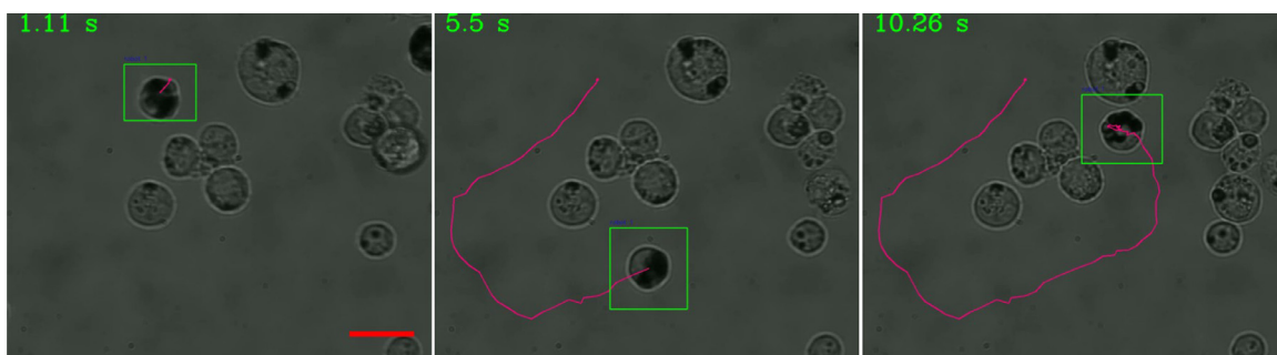
Fig. 12. Trajectory of a synthetically engineered Chinese hamster ovarian cell being manipulated by ingested magnetic microrobots (see Video 2). The micro-robots used were 4.8 \mu\text{m} silica micro-beads coated with 100 nm of Nickel. Scale-bar = 20 \mu\text{m} .
