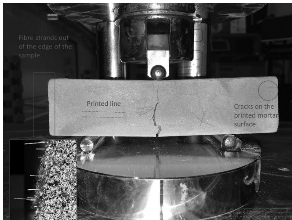
FIG. 9. Prism mortar specimen (160×40×40) mm after being removed from the oven at 90^\circ\text{C} .
