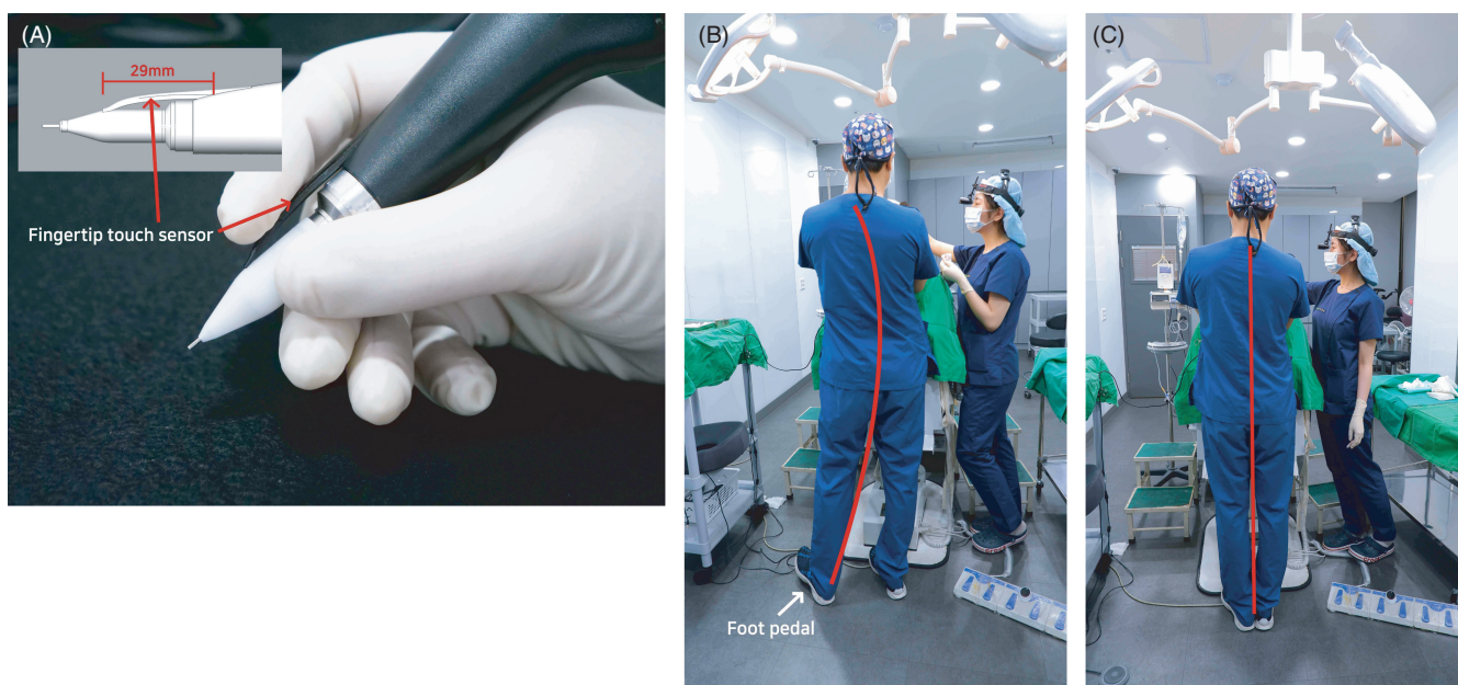
FIGURE 3 Fingertip touch sensor. Fingertip touch sensor: the long extension of the button is convenient as it is activated sensitively by touching anywhere on the rod using the lever principle. For the surgeon using traditional foot pedal switch, standing on one foot induces a non-ergonomic and unstable posture. Using a fingertip touch switch evenly disperses the surgeon's weight and reduces muscle fatigue
