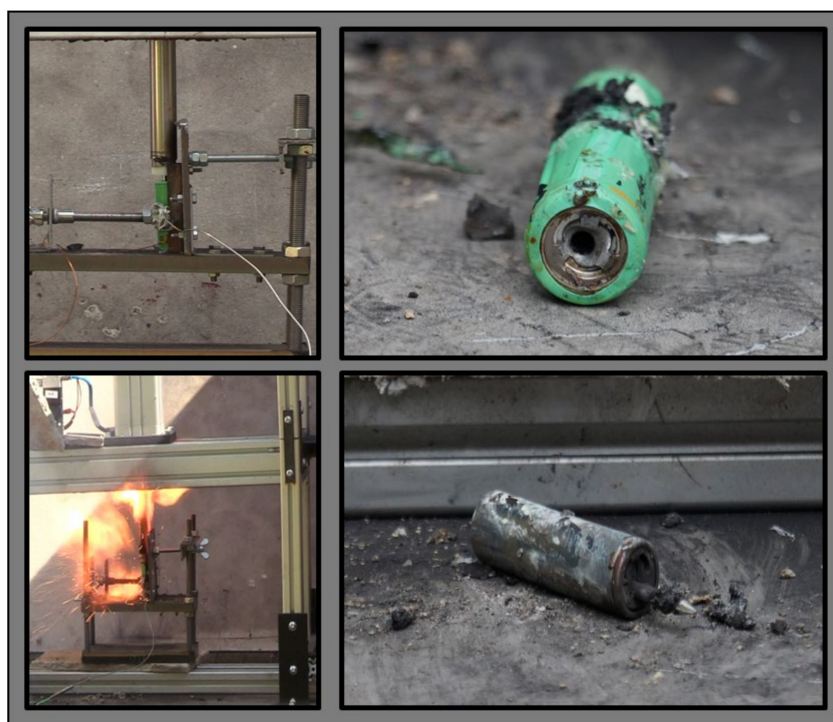
Figure 9. A in \text{CaCl}_2 deactivated cell shows no reaction when the nail penetrates the cell ( top left ); Nail punctured the cell in \text{CaCl}_2 solution in the middle of the positive terminal ( top right ); In DW deactivated cell shows violent reactions when the nail hits the cell ( bottom left ); In DW deactivated cell, which burnt out, nail got stuck in the cell after being pulled out ( bottom right ).
