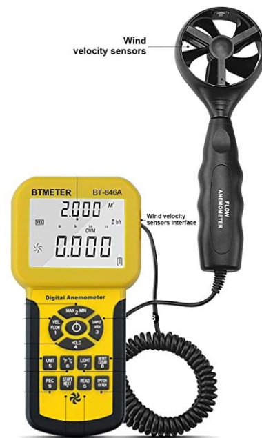
Figure 6. Anemometer: temperature and wind speed sensor.
