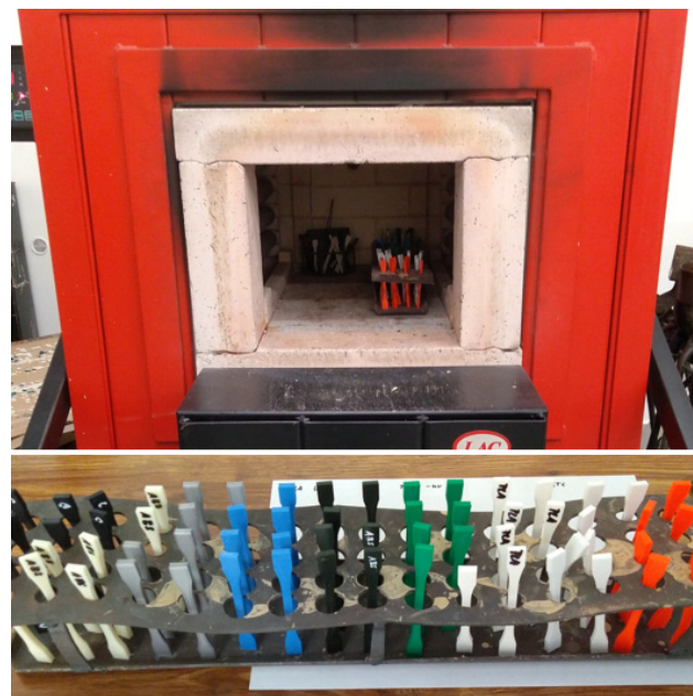
Figure 7. Set of test samples for placing in the furnace.
