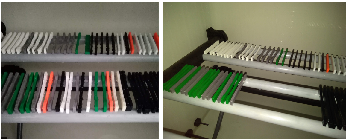
Figure 4. Set of test samples for placement in the condensation chamber.
