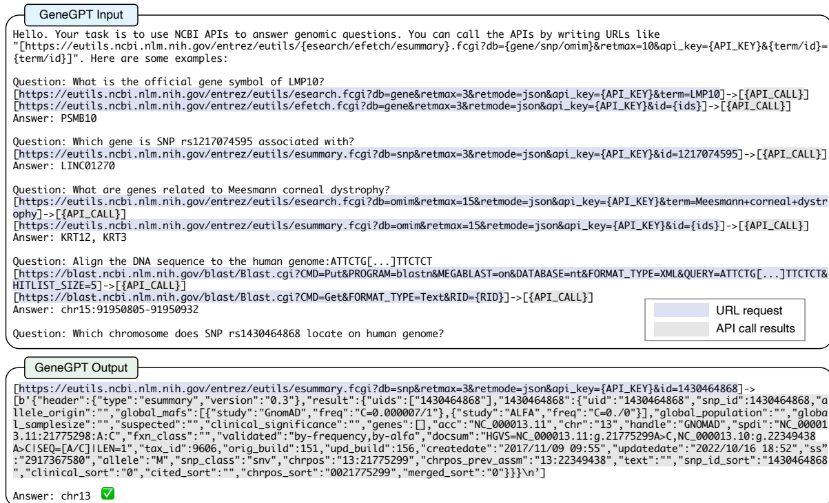
Figure 1: An example of teaching large language models to use NCBI Web APIs and solve genomics questions. The prompt includes three parts: 1. a general task description and an NCBI Web API URL template; 2. Four demonstrations of NCBI API usage (summarized in Table 1); 3. A task-specific test question.
