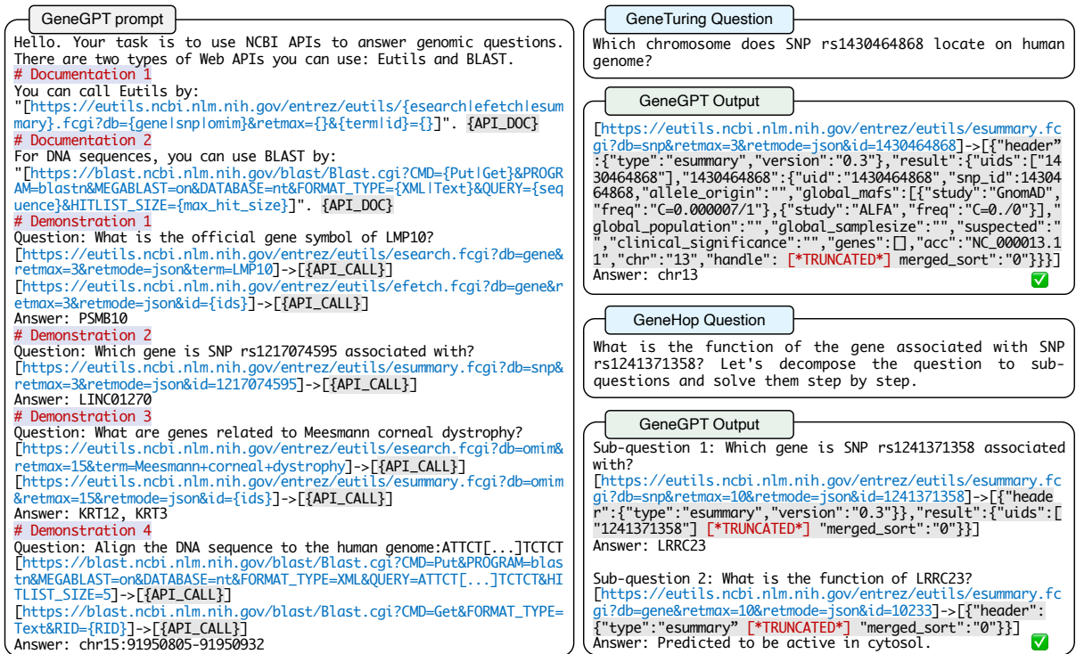
Figure 1: Left: GeneGPT uses NCBI Web API documentations and demonstrations in the prompt for in-context learning. Right: Examples of GeneGPT answering GeneTuring and GeneHop questions with NCBI Web APIs.
