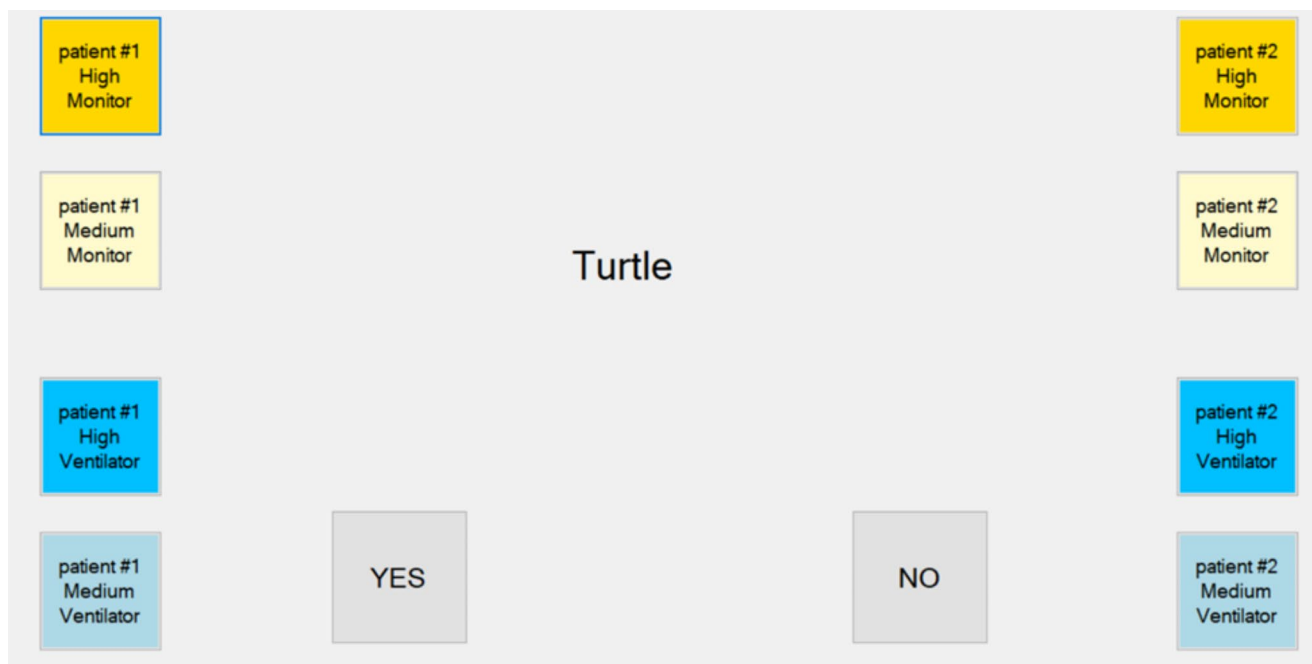
Fig. 2 User interface: On the left are the patient 1 alarms, in the middle are the response keys for the cognitive task, and on the right are the patient 2 alarms
