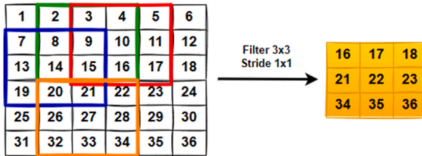
Fig. 5. Max-pooling layer operation with 3 \times 3 filter and 1 \times 1 stride over 6 \times 6 convolved feature is demonstrated to down-sampling of each 3 \times 3 block to map in 1 block (pixel).
