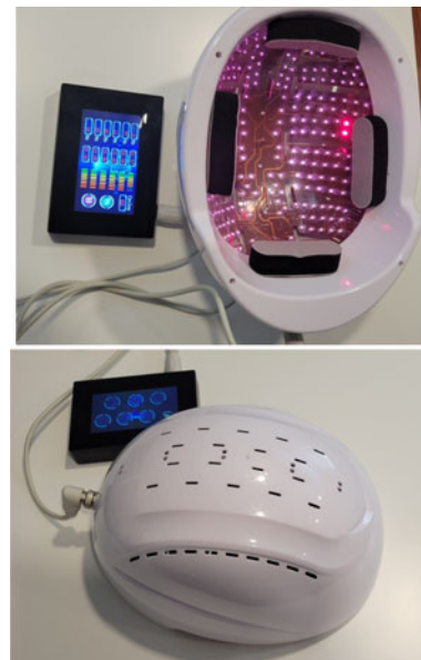
FIG. 2. LED PBM Helmet. LED PBM helmet containing 256 individual LED lights delivering near-infrared (810 nm) wavelength with a power of 60 mW per LED light, for a total power of 15 W, an irradiance of 24 \text{ mW/cm}^2 , energy of 72 Joules, and a fluence of 28.8 \text{ J/cm}^2 was applied to the whole brain for 20 min, while traditional speech-language therapy was provided. LED, light-emitting diode; PBM, photobiomodulation.
