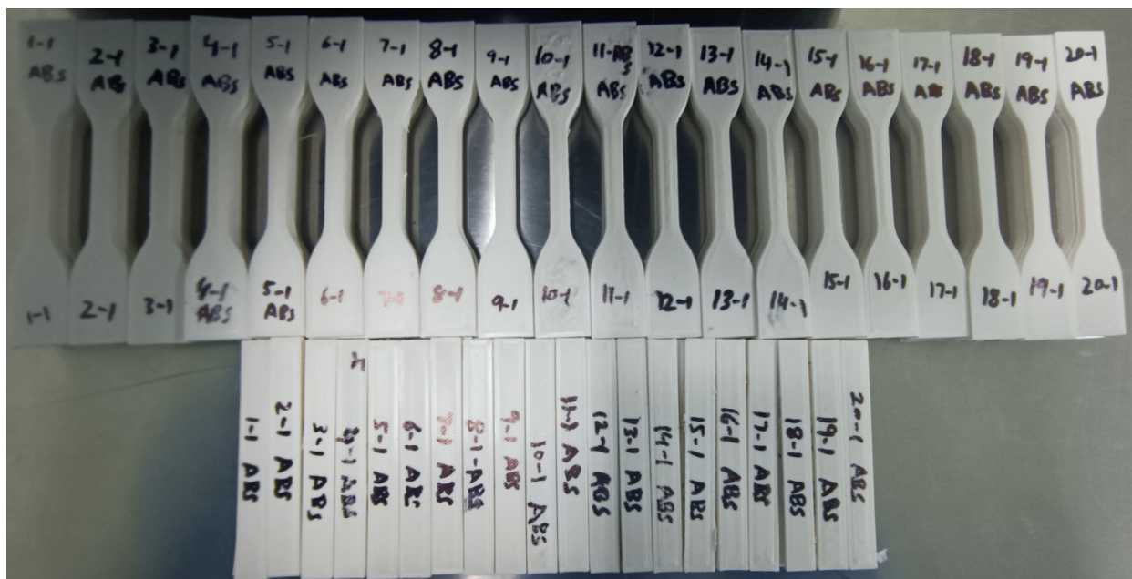
Figure 2. FFF fabricated experimental samples for the ABS polymer.
