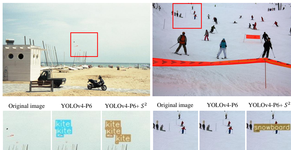
Figure 6. Comparison of bounding box results for small objects between YOLOv4-P6 and the proposed scheme on MS COCO dataset.
