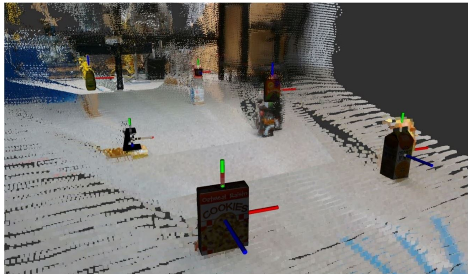
Figure 5. Manually adjusted labeled map with object mesh and pose markers from DOPE fused with RTAB-Map point cloud.
