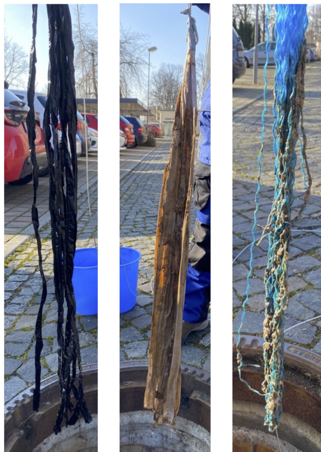
Fig. 2. Passive samplers used for the detection of SARS-CoV-2 GC in wastewater at district-scale level. From left: polyethylene-based plastic sampler, cotton-cloth sampler and unravelled polypropylene plastic rope sampler.
