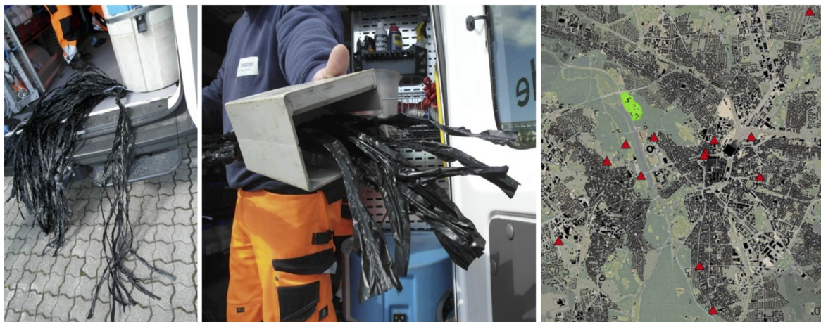
Fig. 1. Polyethylene-based plastic passive samplers used for the detection of SARS-CoV-2 GC in wastewater (left and middle photos), and the location of the 13 passive samplers (red) across the city of Leipzig. Green: Location of the WWTP.
