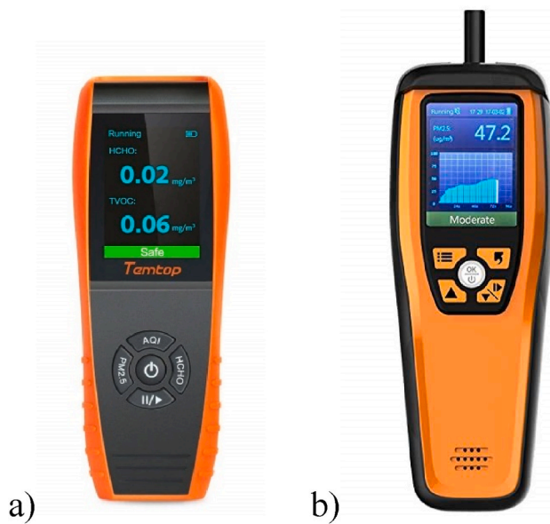
Fig. 10. Air quality monitors used: a) Temptop 1000s+, b) Temptop M2000.
