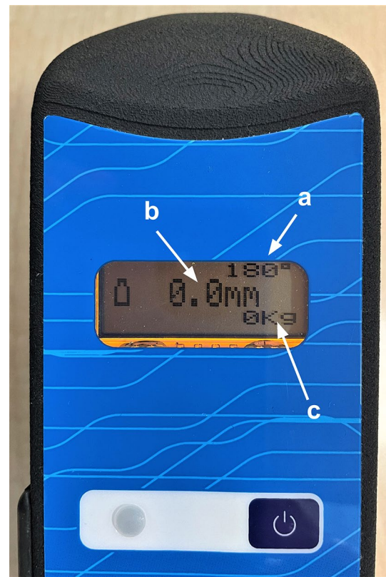
Fig. 2 Digital display of the BLU-DAT device. On the display is possible to visualize knee flexion angle (a), where 180° corresponds to the plane parallel to the ground; anterior tibial translation expressed in mm (b); and the force applied expressed in kilograms (c)
