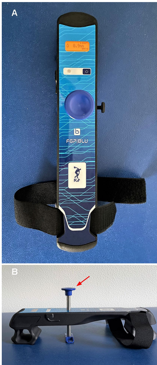
Fig. 1 The BLU-DAT laxity testing device (A). Displacement on the sagittal plane is measured by a magnetic linear encoder whose mobile part is applied to a sliding rod enveloped in a guiding probe (arrow), which is attached to the body of the arthrometer (B)
