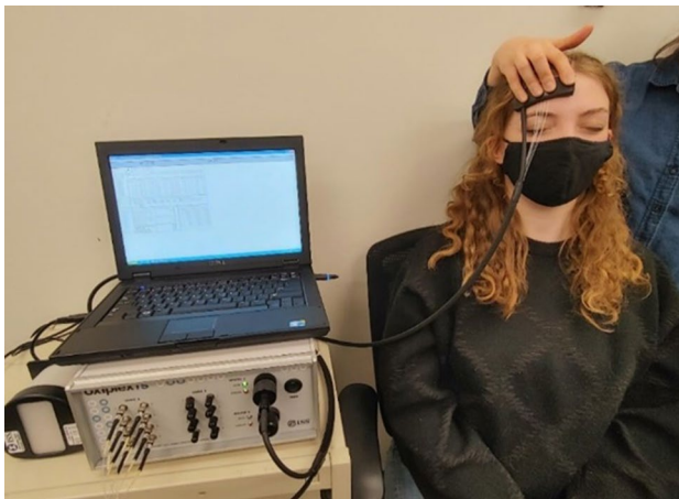
Fig. 1 Frequency-domain near-infrared spectroscopy (ISS OxiplexTS, model 96,208, ISS Inc., Champaign, IL) used in the measurement of frontal cortical microvascular oxygenation ( S_tO_2 )
