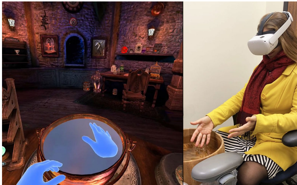
Figure 3. Mixed Reality. VR + real water. While wearing the Meta Quest2 VR HMD, using camera based hand tracking, any movements of the participant's real hands or fingers in the real world are seen by the healthy volunteer participants in the virtual world. During the mixed reality condition, when their virtual hand went into a bowl of animated water in VR (left image), their real hand simultaneously went into a carefully positioned bowl of real water designed to give the computer generated virtual water tactile qualities (image on the right, right image copyright Hunter Hoffman, UW, https://www.vrpain.com ). The image on the left is from the Waltz of the Wizards by Aldin Dynamics, Reykjavik, Iceland, https://www.aladin.io/ , still shot copyright Hunter Hoffman, UW, https://www.vrpain.com ).
