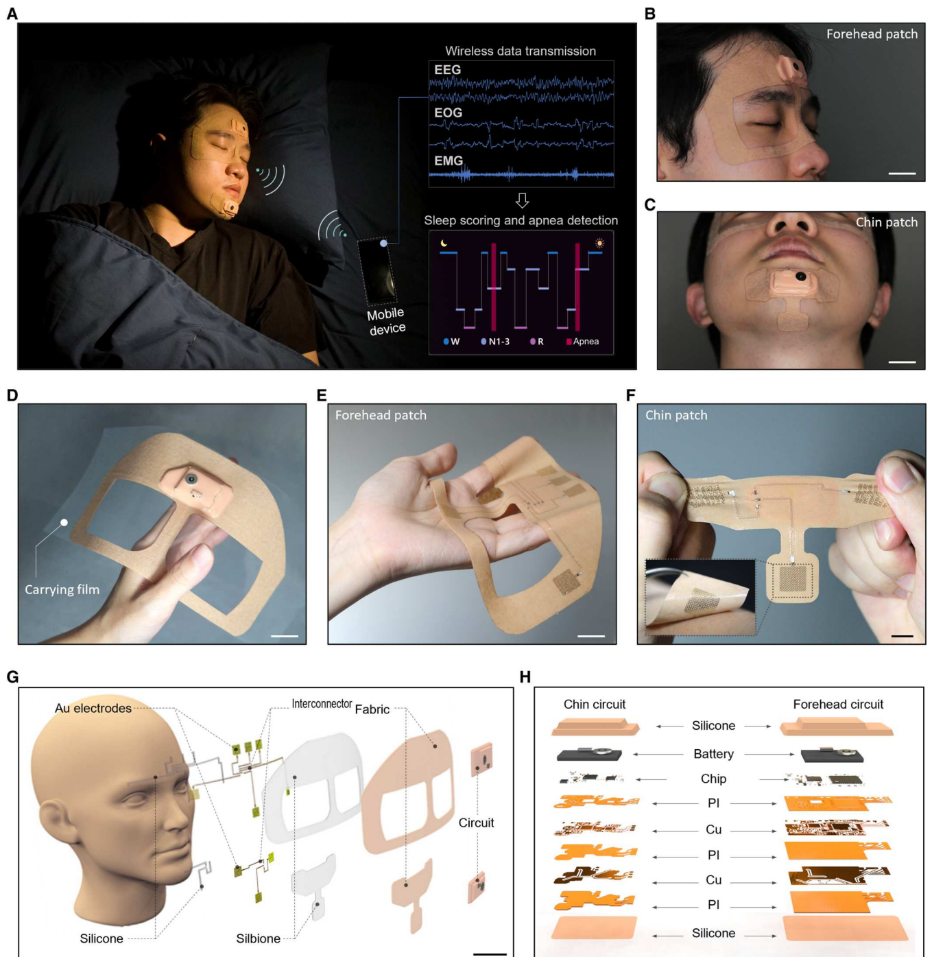
Fig. 1. At-home sleep monitoring patches for assessing sleep quality and sleep apnea. (A) Image of an at-home wireless sleep monitoring system for real-time, multichannel recording of EEG, EOG, and EMG signals and deep learning–based classification of sleep stages and sleep apnea detection using a portable device. (B and C) Photos of the soft wearable patches conformally attached to the facial area, including the forehead (B) and the chin (C). Scale bars, 2 cm. (D) Photo of the forehead patch on a device carrier made of PTFE for convenient handling and storage for multiday uses. Scale bar, 2 cm. (E) Photo of the backside of the highly flexible soft patch in (D) showing nanomembrane electrodes. Scale bar, 2 cm. (F) Photo of the chin patch showing its stretchability to make conformal lamination to the skin (inset image). Scale bar, 1 cm. (G) Illustration of the sleep monitoring system mounted on the face, including electrodes, interconnectors, circuits, and adhesive (Silbione) on a fabric. Scale bar, 3 cm. (H) Details of the multilayered flexible circuits, made of metals, polymers, and chips, which are fully encapsulated by silicone membranes for strain isolation during device assembly, handling, and wearing during sleep.
