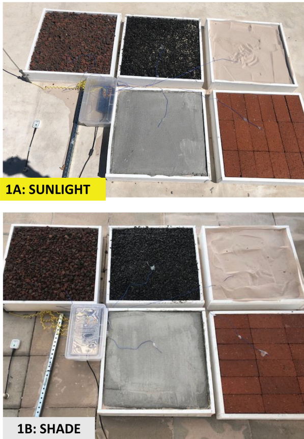
Figure 1. Photographs of experimental data collection set up in direct sunlight (top) and in shade (bottom). This arrangement was placed on the roof of the Thomas T. Beam Engineering Complex on the campus of University of Nevada Las Vegas. Six different material samples were arranged including porous rock (top left), asphalt (top middle), sand (top right), galvanized metal (bottom left), concrete (bottom middle), and brick (bottom right). All but the galvanized metal were placed in a wooden form measuring 2' x 2' and 3.5 inches high. Thermocouples were placed on the surface of each material and held in place with adhesive. Sunlight intensity was measured using a pyranometer which is seen in the lower left corner to the left of the galvanized metal.
